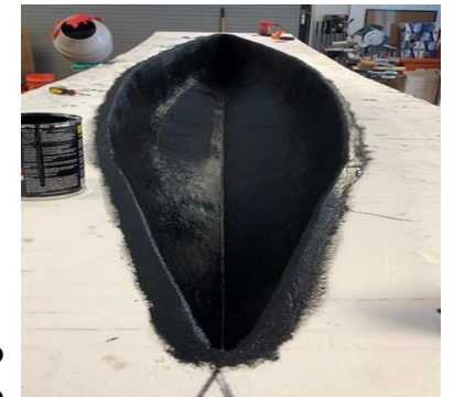
Figure 8: Flex Seal Applied on Mold
