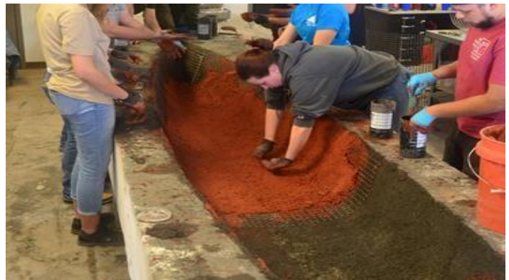
Figure 11: Body Reinforcement and Interior Finishing Layer
